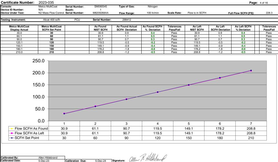
All instruments have been calibrated against standards traceable to NIST. This Certification Sheet must not be altered in any way!
